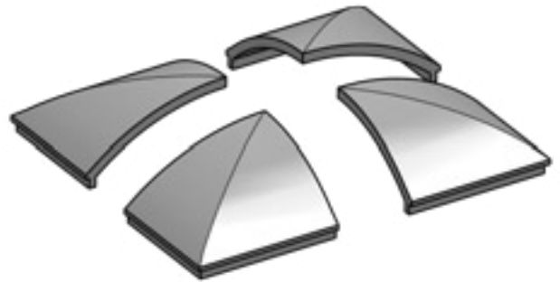
Cross-vault roof shape – CONCEPT-DA-CROSS
